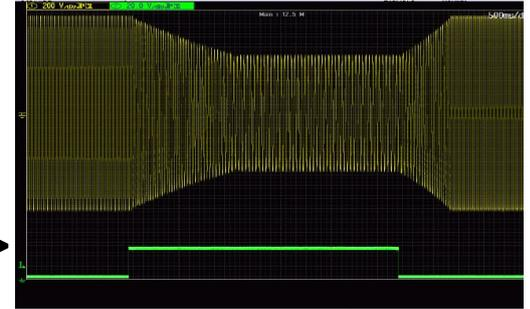
Example for change from 50Hz / 400V to 30Hz and 240V with ramp-down of 2 cycles /Hz and ramp-up of 1 Cycle/Hz. Yellow: output voltage and Green: Mid-Power input signal
