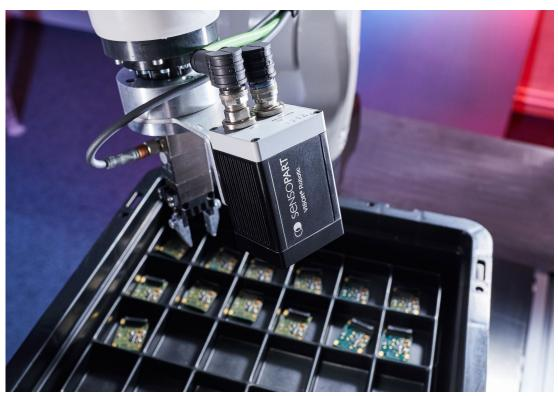
It represents a major technical advancement: In comparison to SensoPart's previous high-end sensor series VISOR® V20 with  $1440 \times 1080$  pixels, the new VISOR® V50 series offers a resolution that is three times bigger:  $2560 \times 1936$  pixels. These sensors achieve an image quality that was previously only available with expensive, complex vision systems; the potential applications of the user-friendly vision sensors have consequently been considerably expanded.
