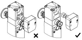
Warning: Despite the fact that the device has been designed to help alignment between the head and the respective actuator, excessive misalignment could cause the actuator to be damaged. Periodically check the alignment between the switch and the respective actuator.
