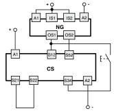
Connections with CS AT-0---- / CS AT-1---- safety modules
