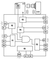
tween the safe outputs (OS1 and OS2) or a short circuit of an output towards earth or towards the power supply. Also in this case, function f3 deactivates the safe outputs, and the error status is in-dicated by the OUT led red blinking light. The O3 signalling output is activated during the "RUN" status when the actuator is inserted in the device, regardless of the status of the IS1and IS2 inputs. The status of this output is displayed by means of the ACT led.
