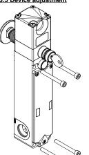
Attention: Once adjustment is complete, retighten the head screws with a torque between 0.8 and 1.2 Nm.
