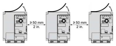
Free space≥50 mm (2 in.) on each side. Vent cover should be removed for operation at surrounding air temperature above 50 °C (122 °F). The degree of protection becomes IP20.
