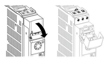
Apply the following instructions to access the power terminals on frame sizes 1B and 2B drives
