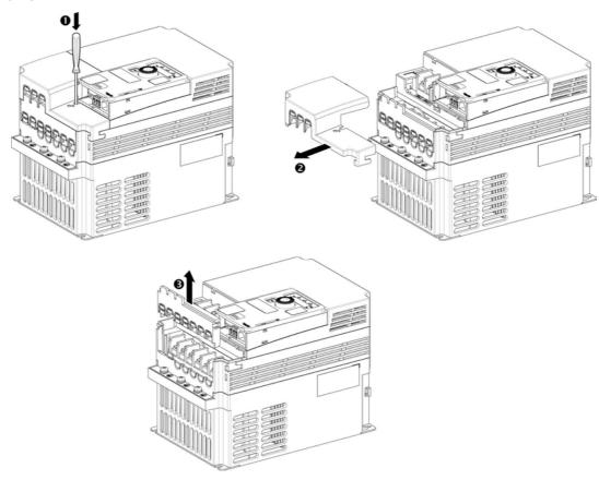
Apply the following instructions to access the power terminals on frame sizes 4C drives
