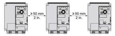
Free space≥50 mm (2 in.) on each side, with vent cover fitted. Mounting type A is suitable for drive operation at surrounding air temperature less or equal to 50 °C (122 °F)
