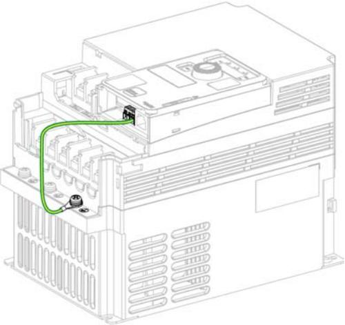
The diagram shows a 3D perspective view of the control block of an ATV320 drive. A green wire is connected to the PE terminal on the top left of the control block. The drive is shown in a partially disassembled state, with the control block cover removed, revealing the internal terminals and components. The drive is mounted on a metal frame, and the PE terminal is located on the top left side of the control block.
