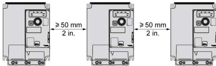
Free space  $\geq 50$  mm (2 in.) on each side, with vent cover fitted. Mounting type A is suitable for drive operation at surrounding air temperature less or equal to 50 °C (122 °F)
