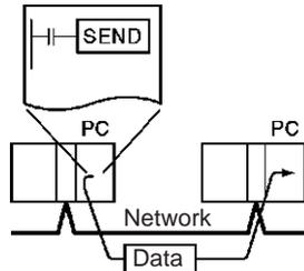
**Transmission to a Host Computer Connected through Host Link**
