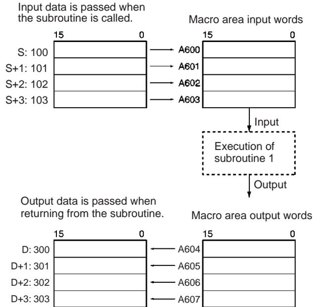
The second MCRO(099) instruction operates in the same way, but the input data in CIO 200 to CIO 203 is passed to A600 to A603 and the output data in A604 to A607 is passed to CIO 400 to CIO 403.
