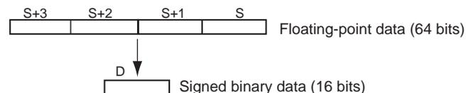
Only the integer portion of the floating-point data is converted, and the fraction portion is truncated. The integer portion of the floating-point data must be within the range of -32,768 to 32,767.
