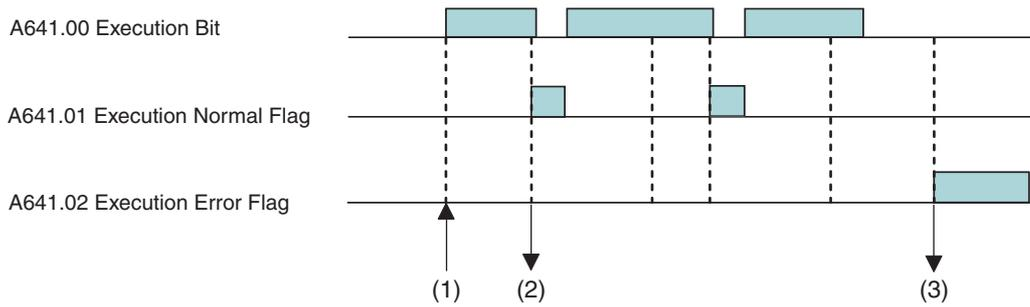
(1) Turn ON A641.00 (Execution Bit) to send command data stored starting at D1300. For details, refer to *DM Area Data* on page 14-19.
