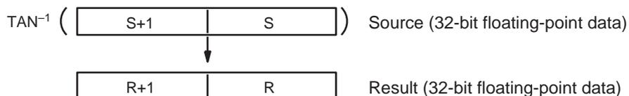
The result is output to words R+1 and R as an angle (in radians) within the range of  $-\pi/2$  to  $\pi/2$ .
