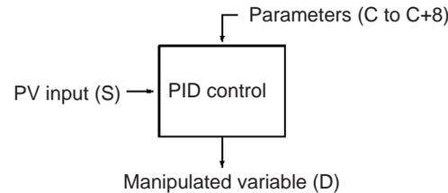
The number of valid input data bits within the 16 bits of the PV input (S) is designated by the input range setting in C+6, bits 08 to 11. For example, if 12 bits (4 hex) is designated for the input range, the range from 0000 hex to 0FFF hex will be enabled as the PV. (Values greater than 0FFF hex will be regarded as 0FFF hex.)
