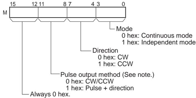
**Note:** Use the same pulse output method when using both pulse outputs 0 and 1 (CP1H only).
