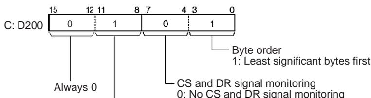
This example assumes that both a start and end code have been specified in the PLC Setup.
