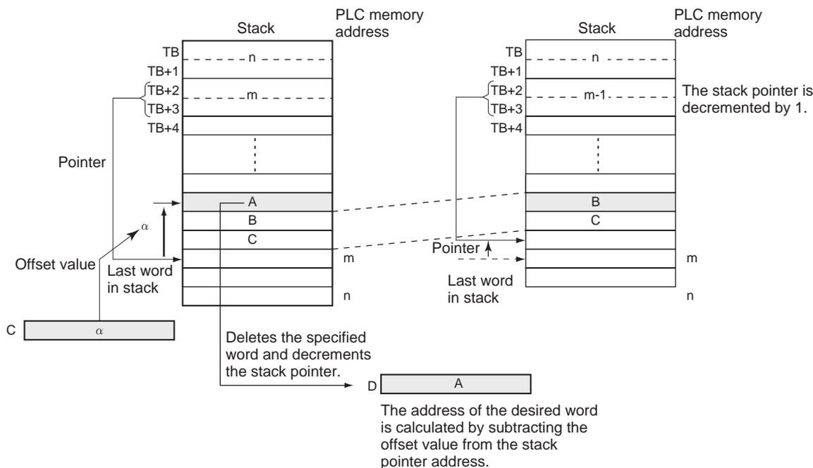
SDEL(642) can be used to delete the data for an item that is rejected from the items on a conveyor. The position of the deletion point is simply the number of items back (the offset value) from the most recent item added to the conveyor.
