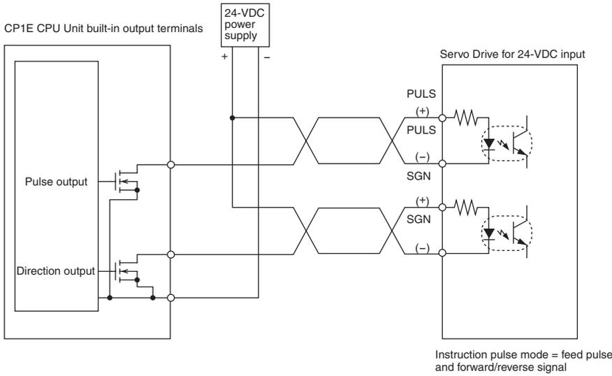
N□□S(1)-type (Example: Sinking outputs)
