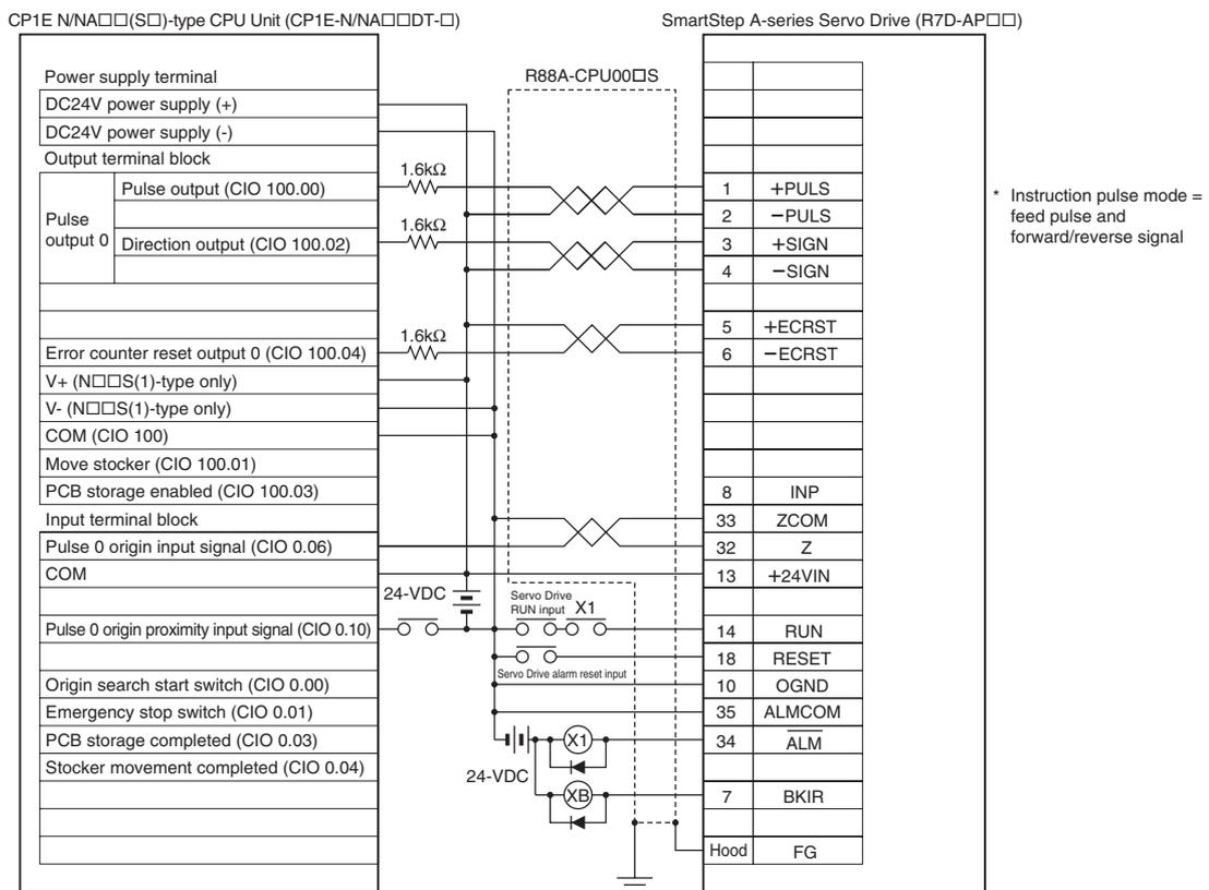
Only N□□S(1)-type CPU Units can wire V+ and V-. Do not wire them in N□□-type CPU Units.
