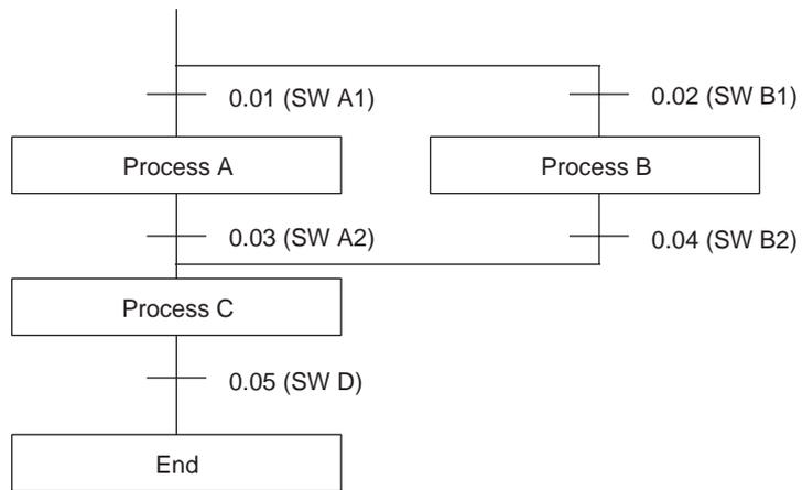
The program for this process, shown below, starts with two SNXT(009) instructions that start processes A and B. Because of the way CIO 0.01 (SW A1) and CIO 0.02 (SW B1) are programmed, only one of these will be executed with an ON execution condition to start either process A or process B. Both of the steps for these processes end with a SNXT(009) that starts the step (process C).
