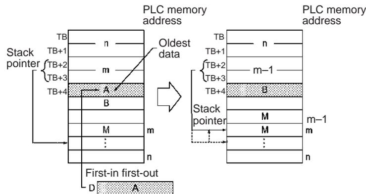
Use FIFO(633) in combination with PUSH(632). After PUSH(632) has been used to write data into a stack, FIFO(633) can be used to read data from the stack on a first-in first-out basis.
