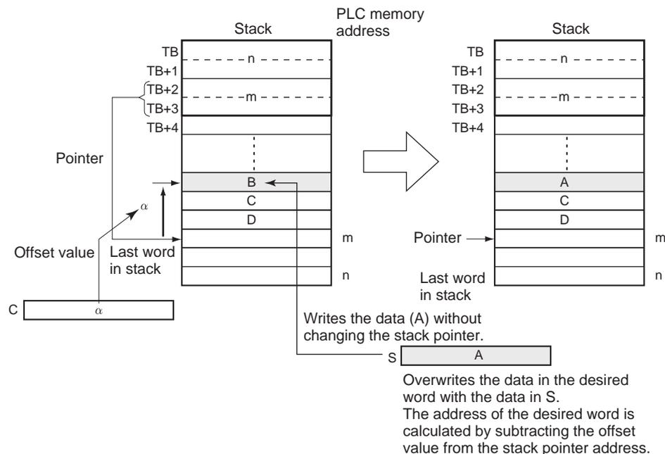
SWRIT(640) can be used to change the data for an item currently on a conveyor. The position of the desired item is simply the number of items back (the offset value) from the most recent item added to the conveyor.
