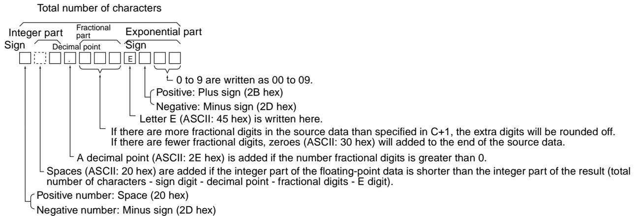
**Note** Either one or two bytes of zeroes are added to the end of ASCII text as an end code.
