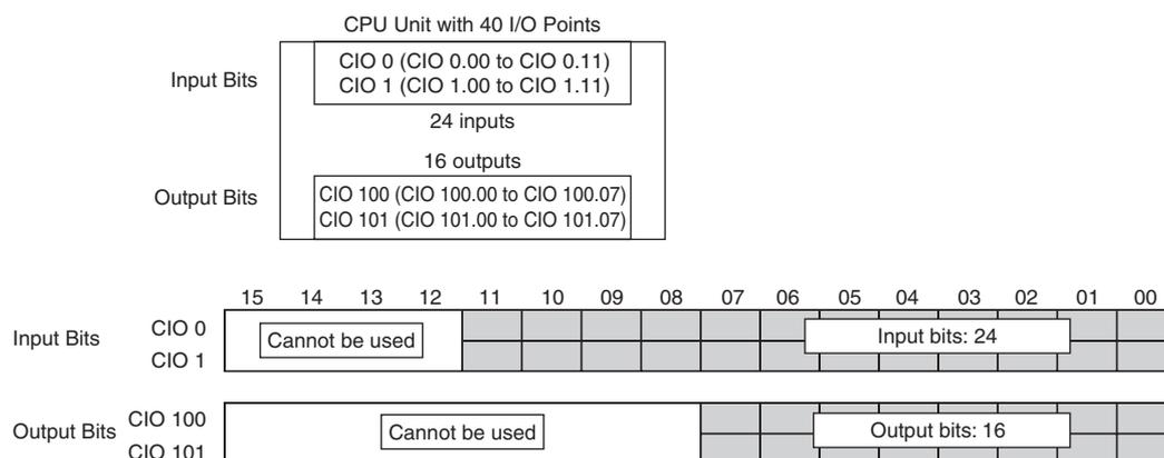
For a CPU Unit with 40 I/O points, a total of 24 input bits are allocated to the input terminal block. The bits that are allocated are input bits CIO 0.00 to CIO 0.11 (i.e., bits 00 to 11 in CIO 0) and input bits CIO 1.00 to CIO 1.11 (i.e., bits 00 to 11 in CIO 1).
