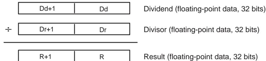
If the absolute value of the result is greater than the maximum value that can be expressed as floating-point data, the Overflow Flag will turn ON and the result will be output as ±∞.
