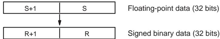
Only the integer portion of the floating-point data is converted, and the fraction portion is truncated. (The integer portion of the floating-point data must be within the range of -2,147,483,648 to 2,147,483,647.)
