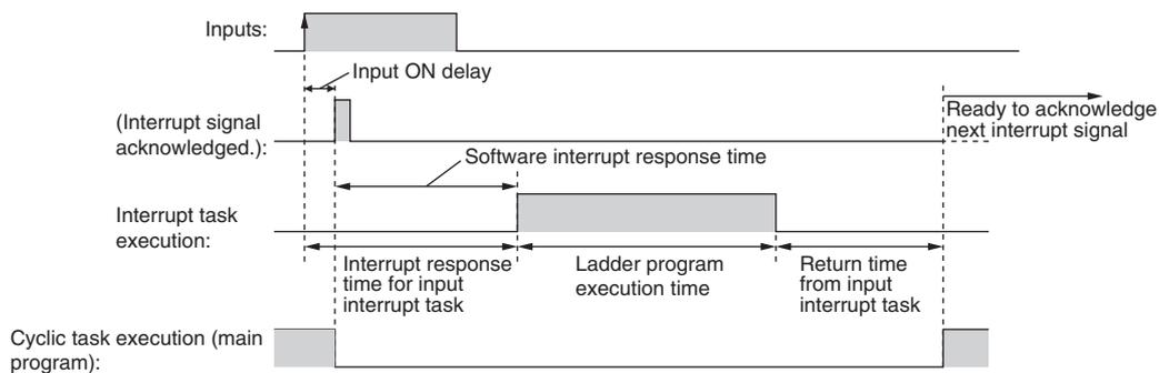
The time from when execution of the input interrupt task is completed until execution of the cyclic task is resumed is 24  $\mu$ s.
