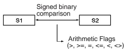
**Note** CPS(114) treats the data in S<sub>1</sub> and S<sub>2</sub> as signed binary data which ranges from 8000 to 7FFF (-32,768 to 32,767 decimal).
