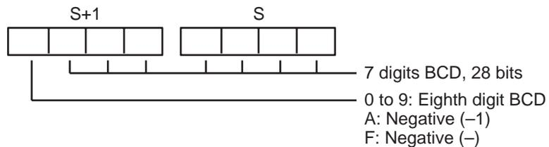
The following table shows the possible double signed binary values for each signed BCD format. An error will occur if the source data is not within the allowed range for the specified signed BCD format.
