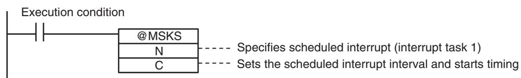
The MSKS instruction must be executed only once to make the settings, so in general execute MSKS in just one cycle using the upwardly differentiated variation of the instruction.
