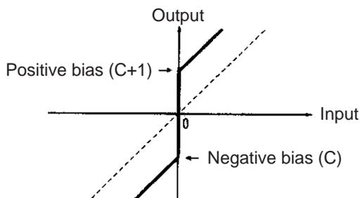
If the output data is smaller than the 8000 (hex) or if is greater than 7FFF, the sign will be reversed. For example, for a negative bias value of FF00 (hex) and input data of 8000 (hex), the output data will be as follows:
