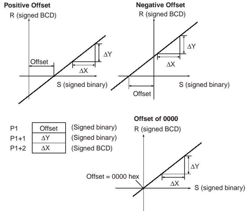
SCL2(486) can be used to scale the results of analog signal conversion values from Analog Input Units according to user-defined scale parameters. For example, if a 1 to 5-V input to an Analog Input Unit is input to memory as 0000 to 0FA0 hexadecimal, the value in memory can be scaled to -100 to 200°C using SCL2(486).
