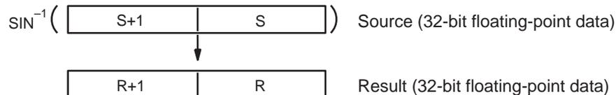
The source data must be between  $-1.0$  and  $1.0$ . If the absolute value of the source data exceeds  $1.0$ , an error will occur and the instruction will not be executed.
