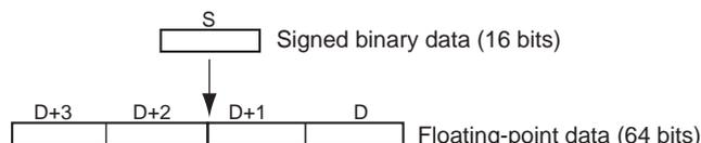
Only values within the range of -32,768 to 32,767 can be specified for S. To convert signed binary data outside of that range, use DBLL(844).
