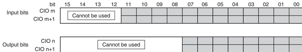
Two input words (24 bits) and two output words (16 bits) are allocated to a 40-point I/O Unit.
