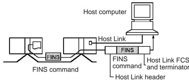
**Serial Gateway Communications to a Component or Host Link Slave**
