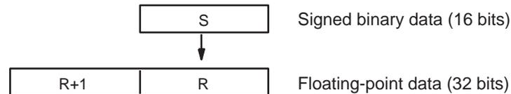
Only values within the range of -32,768 to 32,767 can be specified for S. To convert signed binary data outside of that range, use FLTL(453).
