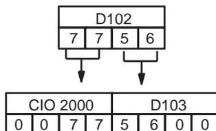
6. If the content of D103 is greater than 4900, CIO 2000 is incremented by 1. In this case, the result is 78.
