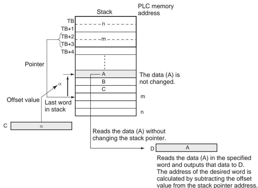
SREAD(639) can be used to read the data for an item currently on a conveyor. The position of the desired item is simply the number of items back (the offset value) from the most recent item added to the conveyor.
