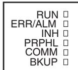
**RUN:** Lit green when the PLC is in RUN or MONITOR mode.
