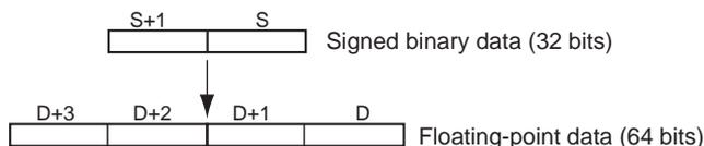
Signed binary data within the range of -2,147,483,648 to 2,147,483,647 can be specified for S+1 and S. The floating point value has 24 significant binary digits (bits). The result will not be exact if a number greater than 16,777,215 (the maximum value that can be expressed in 24-bits) is converted by DBLL(844).
