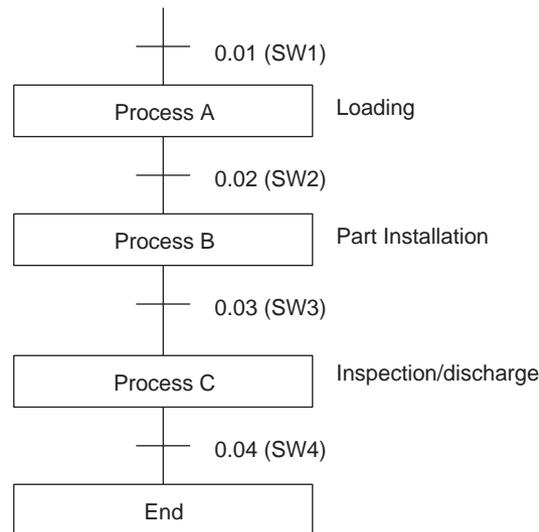
The program for this process, shown below, utilizes the most basic type of step programming: each step is completed by a unique SNXT(009) that starts the next step. Each step starts when the switch that indicates the previous step has been completed turns ON.
