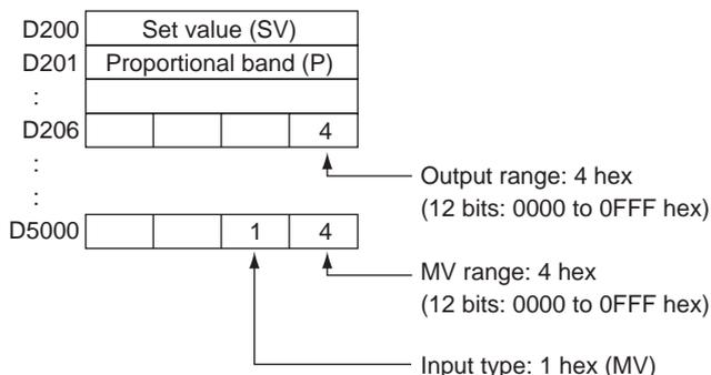
**Note** When using TPO(685) in combination with PID(190) in a cyclic task and also using an interrupt task, temporarily disable interrupts by executing DI(693) (DISABLE INTERRUPTS) ahead PID(190) and TPO(685). If interrupts are not disabled and an interrupt occurs between the PID(190) and TPO(685), the control period may be shifted.
