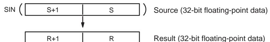
Specify the desired angle (–65,535 to 65,535) in radians in S+1 and S. If the angle is outside of the range –65,535 to 65,535, an error will occur and the instruction will not be executed. For information on converting from degrees to radians, see 3-14-19 LOGARITHM: LOG(468) DEGREES-TO-RADIANS: RAD(458).
