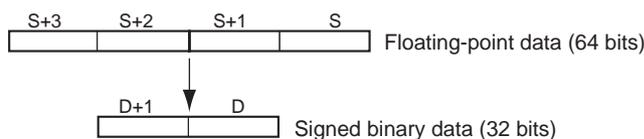
Only the integer portion of the floating-point data is converted, and the fraction portion is truncated. (The integer portion of the floating-point data must be within the range of -2,147,483,648 to 2,147,483,647.)
