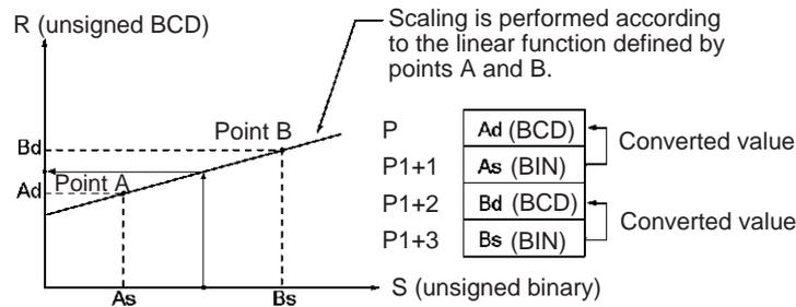
SCL(194) can be used to scale the results of analog signal conversion values from Analog Input Units according to user-defined scale parameters. For example, if a 1 to 5-V input to an Analog Input Unit is input to memory as 0000 to 0FA0 hexadecimal, the value in memory can be scaled to 50 to 200°C using SCL(194).
