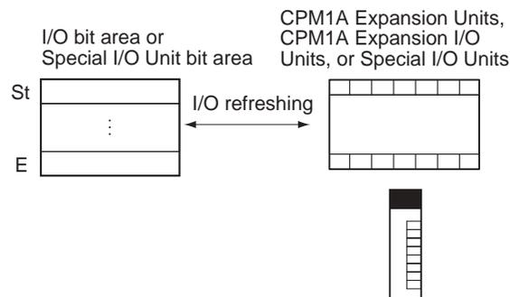
IORF(097) cannot be used for built-in I/O on the CPU Unit or for CPU Bus Units. Use instructions with the immediate refresh option. IORF(097) and immediate refresh options cannot be used for built-in analog I/O on XA CPU Units.
