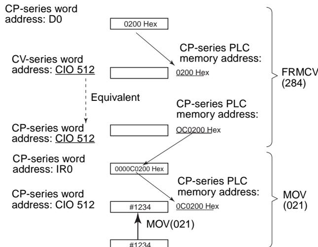
**Example 2: Converting a CV-series Program with PLC Memory Addresses Stored directly in Index Registers**
