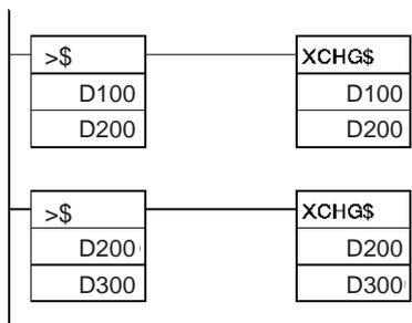
Two text strings beginning with D100 and D200 are compared in ASCII order from lower to higher. If the text string beginning with D100 is higher in ASCII order than the one beginning with D200, then the position of the two text strings will be reversed.
