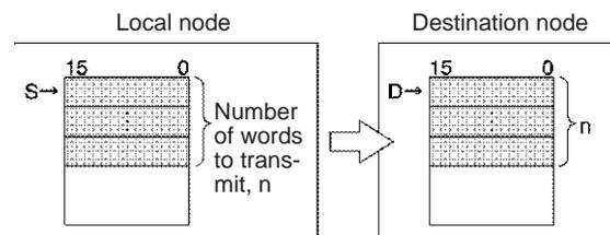
If the destination node number is set to FF, the data will be broadcast to all of the nodes in the designated network. This is known as a broadcast transmission.
