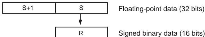
Only the integer portion of the floating-point data is converted, and the fraction portion is truncated. The integer portion of the floating-point data must be within the range of -32,768 to 32,767.
