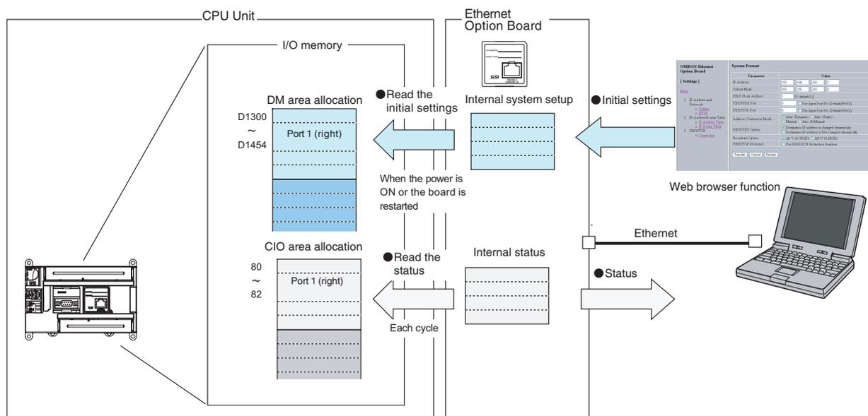
**Note** The initial settings of the Ethernet Option Board cannot be set in the allocated words in the DM area or in the CX-Programmer's system settings.
