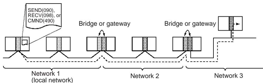
In order to communicate through the network, it is necessary to register a routing table in each PLC's CPU Unit which indicates the route by which data will be transferred to the desired node. Each routing table is made up of a local network table and a relay network table.
