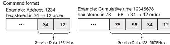
The following diagrams show how data is stored in the data areas when the service data is in 2-byte or 4-byte units.
