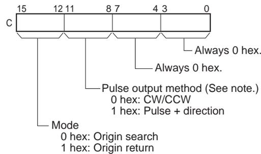
**Note:** Use the same pulse output method when using both pulse outputs 0 and 1.
