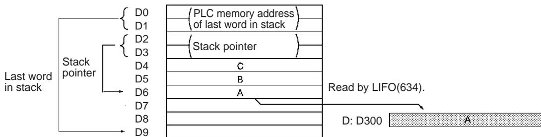
After the data is written to D300, the stack pointer is decremented by one. The content of D6 is left unchanged.
