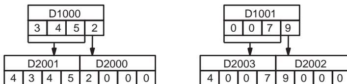
3. FDIV(079) divides the floating-point number in D2001 and D2000 by the floating-point number in D2003 and D2002.
