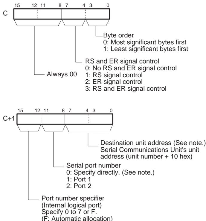
**Note** The serial port's unit address can be specified directly by setting the serial port number to 0 and setting the destination unit address to the serial port's unit address. (Set the destination unit address to 80 hex + 4 × unit number for port 1 or 81 hex + 4 × unit number for port 2.)
