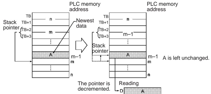
Use LIFO(634) in combination with PUSH(632). After PUSH(632) has been used to write data into a stack, LIFO(634) can be used to read data from the stack on a last-in first-out basis. After data is stored by PUSH(632), the stack pointer indicates the address next to the last data.
