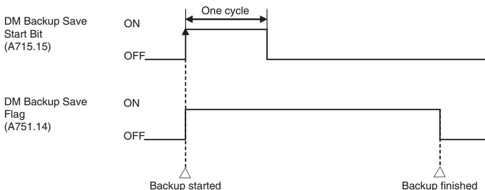
When the saving operation has been completed, A751.14 (DM Backup Save Flag) will turn OFF.
