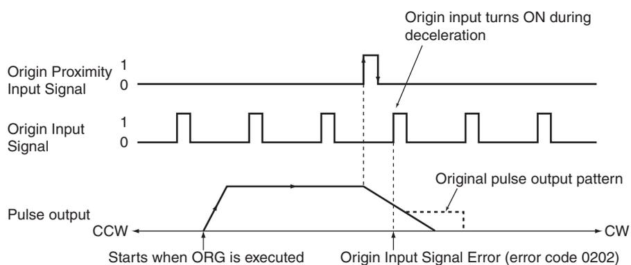
**● Operating Mode 1 (with Error Counter Reset Output, without Positioning Completed Input)**
