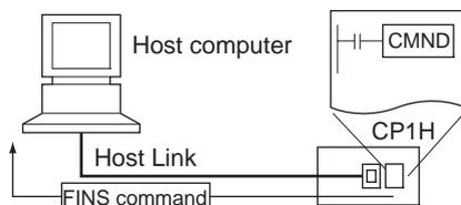
CMND(490) can be executed for either port on the CPU Unit (Serial Communications Option Boards) or CJ-series Serial Communications Unit to send a command to the connected host computer. (Specify the serial port as 1 hex or 2 hex in bits 08 to 11 of C+2.) The command is a FINS message enclosed between a host link header and terminator. Any FINS command can be sent; the host link header code is 0F hexadecimal.
