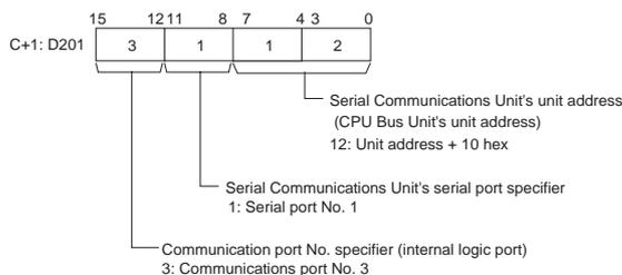
**Note:** The Serial Communications Unit's serial port unit address can also be directly specified in C+1.
