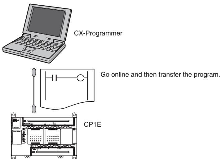
**1** Open the project containing the program to be transferred from the CX-Programmer.
