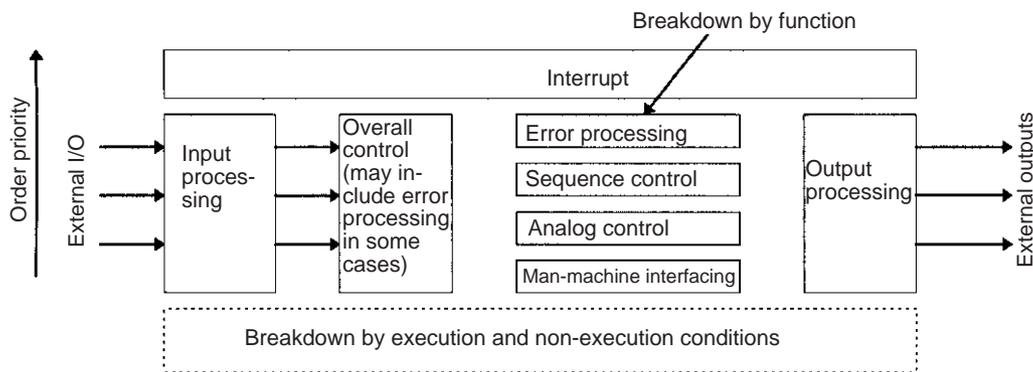
2. Be sure to break down and design programs in a manner that will ensure autonomy and keep the amount of data exchanged between tasks (programs) to an absolute minimum.
