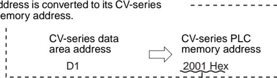
3. The CV-series PLC memory address is stored in D.
