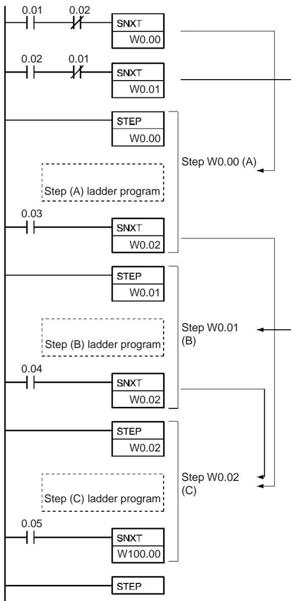
The above programming is used when steps A and B cannot be executed simultaneously. For simultaneous execution of A and B, delete the execution conditions illustrated below.
