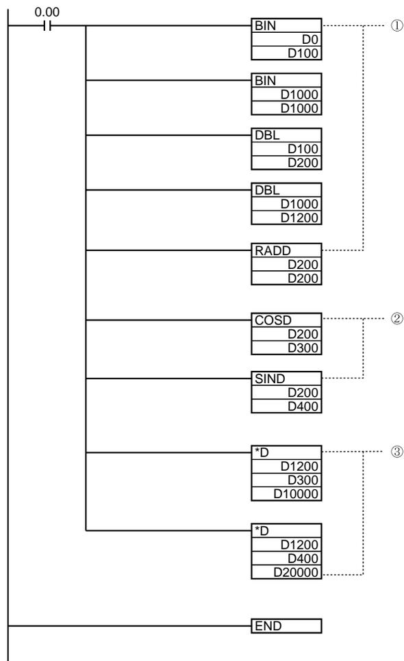
1. This program section converts the BCD data to single-precision floating-point data (32 bits, IEEE754-format).
