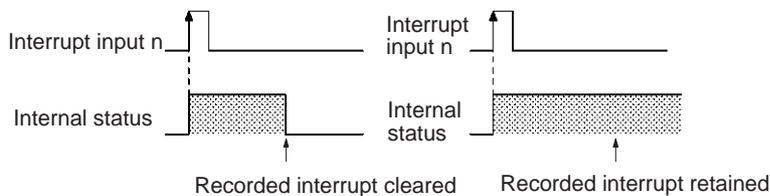
If an input interrupt task is being executed and an interrupt input with a different interrupt number is received, that interrupt number is recorded internally. The recorded input interrupts are executed later in order of their priority (from the lowest number to the highest). CLI(691) can be used to clear these recorded interrupts before they are executed.
