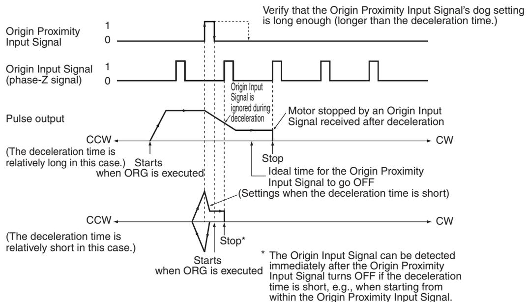
**Operating Mode 1 without Origin Proximity Input Signal Reverse (Origin Detection Method Setting = 1)**
