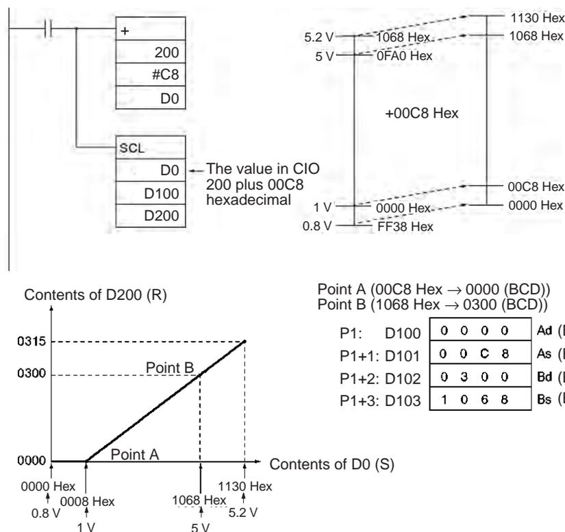
In this example, values from 0000 to 00C8 hexadecimal will be converted to negative values. SCL(194), however, can output only unsigned BCD values from 0000 to 9999, so 0000 BCD will be output whenever the contents of D0 is between 0000 and 00C8 hexadecimal.
