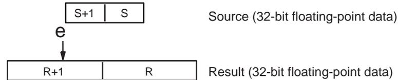
If the absolute value of the result is greater than the maximum value that can be expressed as floating-point data, the Overflow Flag will turn ON and the result will be output as  $\pm\infty$ .
