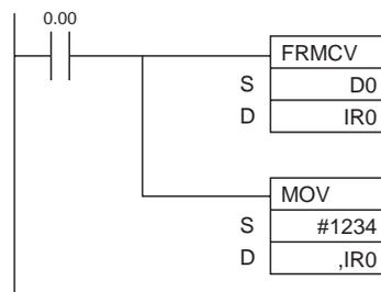
In this case, the value in D0 is 200 hex. The corresponding CV-series data area address is CIO 512. The CP-series PLC memory address for CIO 512 is 0000C200 hex, so this value is stored in IR0. The destination operand in MOV(021) indirectly addresses the content of IR0, so #1234 is transferred to CIO 512.
