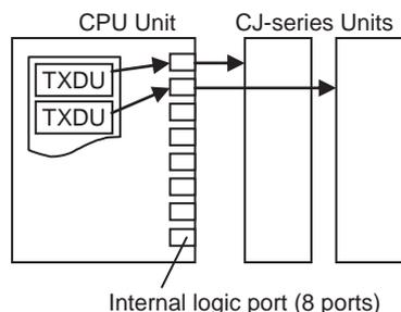
TXDU(256) can not be executed while the TXDU Instruction Executing Flag (bit 5 of n+9 or n+19, where n = CIO 1500 + 25 × unit number) is ON. To ensure that another TXDU(256) is not executed for the port before the first TXDU(256) is completed, program the port's TXDU Instruction Executing Flag as a normally closed condition.
