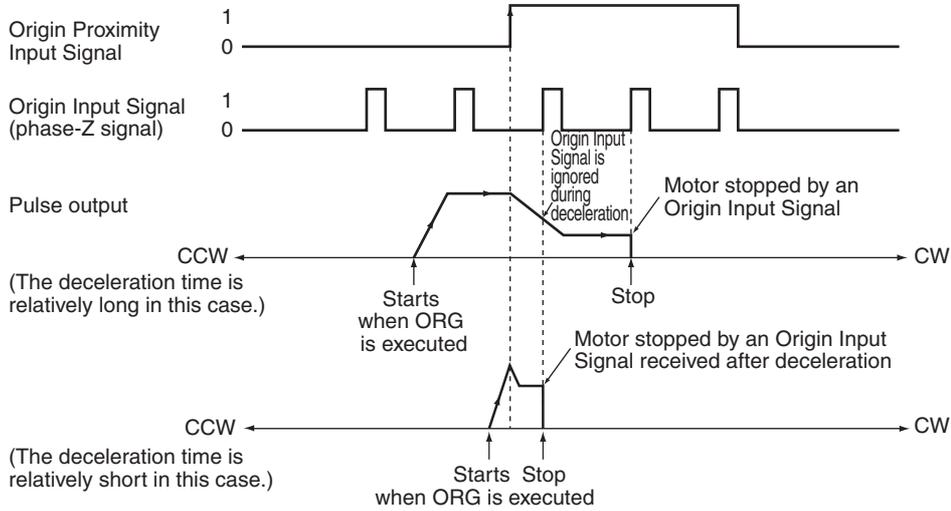
● **Operating Mode 2 (with Error Counter Reset Output, with Positioning Completed Input)**
