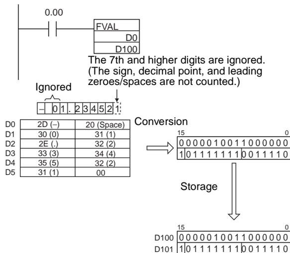
**Converting ASCII Text in Scientific Notation**
