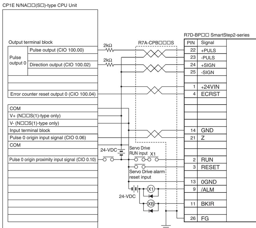
Only N□□S(1)-type CPU Units can wire V+ and V-. Do not wire them in N□□-type CPU Units.
