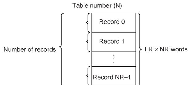
The two record-table instructions associated with DIM(631) are SETR(635) and GETR(636). SETR(635) sets the leading PLC memory address of the specified record number in the specified Index Register. GETR(636) outputs the record number of the record that includes the specified Index Register value (PLC memory address).
