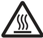
The triangle symbol indicates precautions (including warnings). The specific operation is shown in the triangle and explained in text. This example indicates a precaution for hot surfaces.
