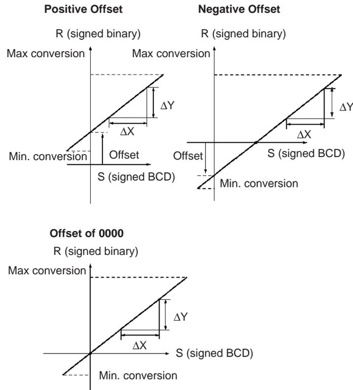
SCL3(487) is used to convert data using a user-defined scale to signed binary for Analog Output Units. For example, SCL3(487) can convert 0 to 200 °C to 0000 to 0FA0 (hex) and output an analog output signal 1 to 5 V from the Analog Output Unit.
