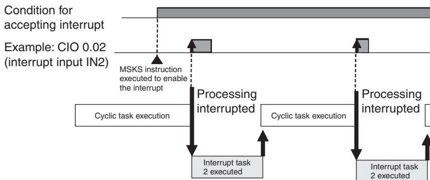
The pulse widths of interrupt input signals must meet the following conditions.
