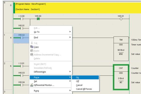
The input bit will be force-set. A symbol indicating the force-set status will be displayed at the input condition.
