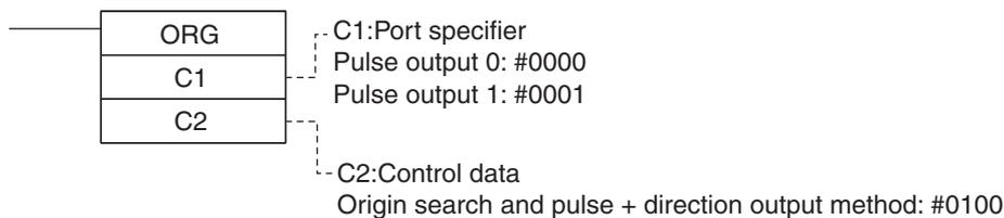
**Note** An instruction execution error will occur if the origin is not defined (relative coordinate system) when the ORG instruction is executed to perform an origin return operation.
