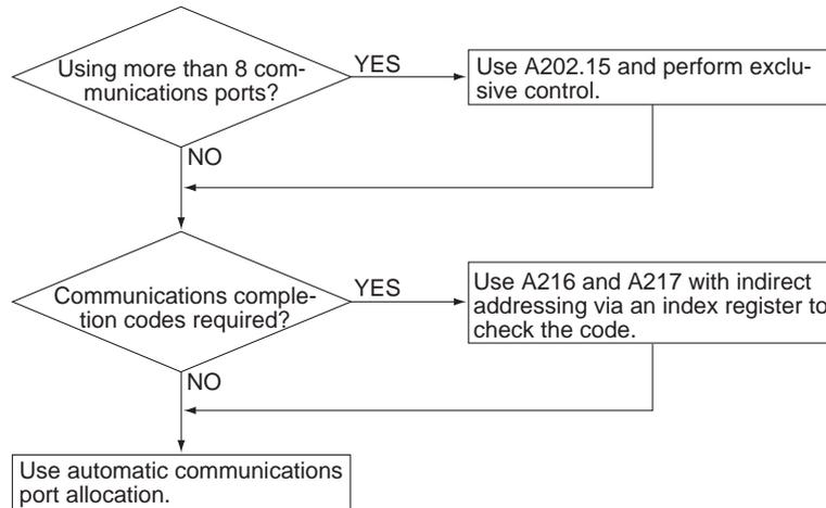
(2) The Auxiliary Area bits and words used for user-specified communications ports are listed in the following table.
