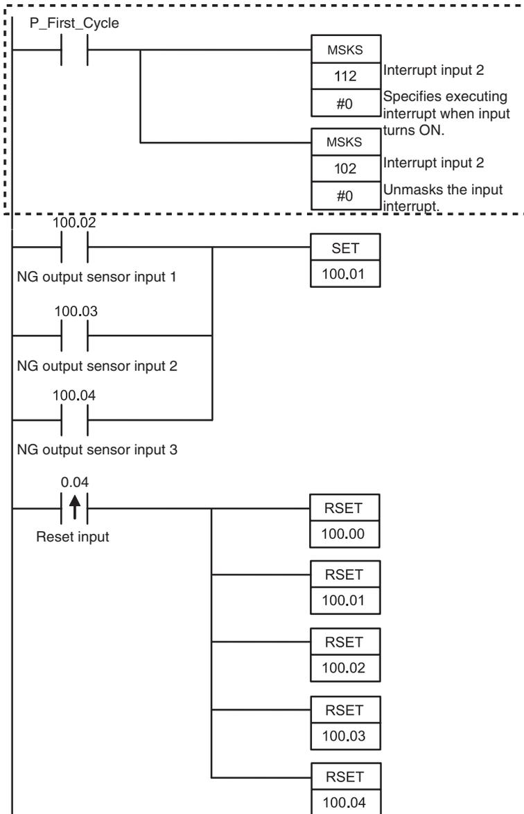
The MSKS instruction is used to specify an interrupt when the input turns ON and then it is used to unmask the input interrupt.
