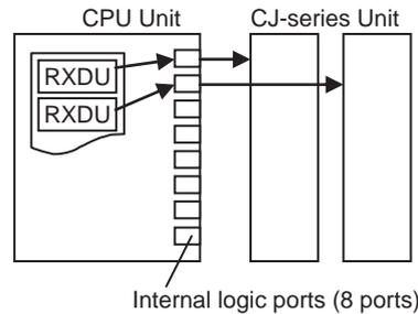
RXDU(255) can not be executed while the Reception Completed Flag (bit 6 of n+9 or n+19, where n = CIO 1500 + 25 × unit number) is ON. Program the Reception Completed Flag as a normally open condition of RXDU(255).
