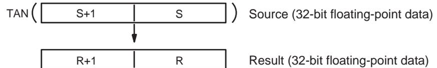
Specify the desired angle (-65,535 to 65,535) in radians in S+1 and S. If the angle is outside of the range -65,535 to 65,535, an error will occur and the instruction will not be executed. For information on converting from degrees to radians, see 3-14-9 DEGREES TO RADIANS: RAD(458).
