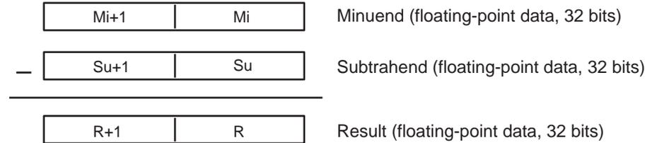
If the absolute value of the result is greater than the maximum value that can be expressed as floating-point data, the Overflow Flag will turn ON and the result will be output as  $\pm\infty$ .
