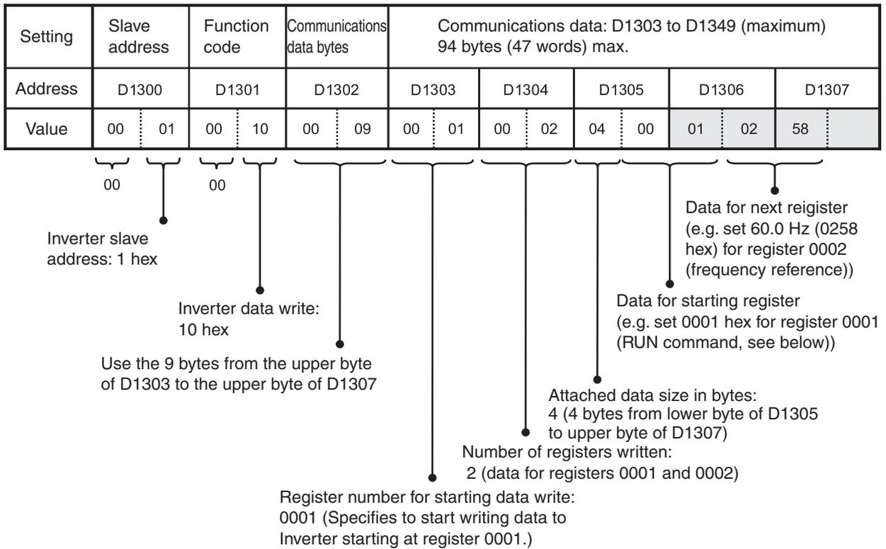
**RUN Command (Register 0001) Allocation and Details for Inverter 3G3MV**
