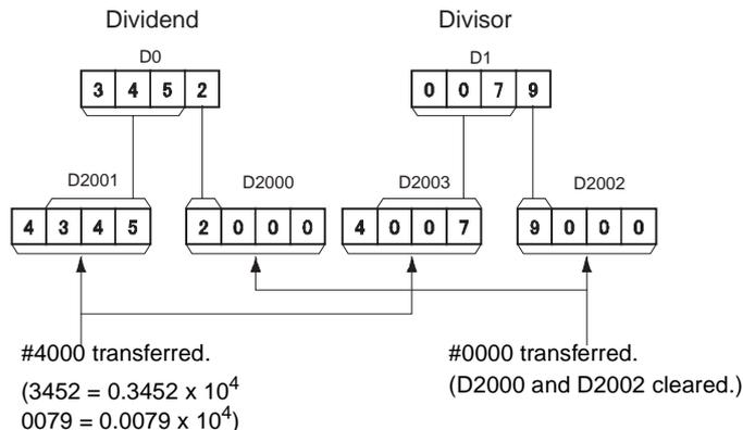
2. MOVD(083) is used to move the digits of the original source words to the proper digits in the 2-word floating-point formats.
