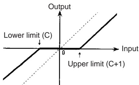
If the output data is smaller than the 8000 (hex) or if is greater than 7FFF, the sign will be reversed. For example, for a lower limit of 0100 (hex) and input data of 8000 (hex), the output data will be as follows:
