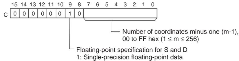
If 16-bit binary or BCD data is being used, the line-segment data is contained in words C+1 through C+2m+2. If 32-bit binary or floating point data is being used, the line-segment data is contained in words C+1 through C+4m+4.
