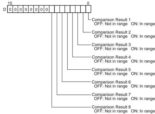
■ **Reading Pulse Output or High-speed Counter Frequency (C = 00□3 hex)**
