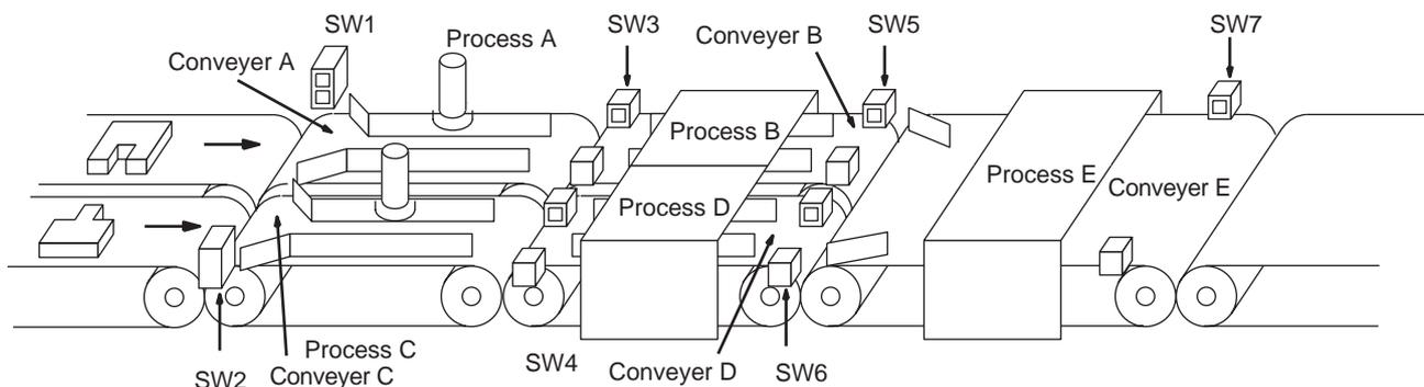
The following diagram demonstrates the flow of processing and the switches that are used for execution control. Here, process A and process C are started together. When process A finishes, process B starts; when process C finishes, process D starts. When both processes B and D have finished, process E starts. E starts.
