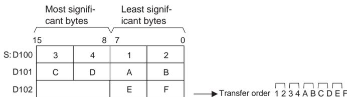
Example allocated DM Setup Area settings:
