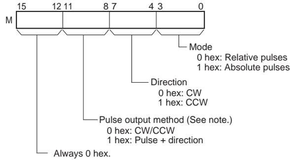
**Note:** Use the same pulse output method when using both pulse outputs 0 and 1.
