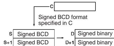
When the converted data is negative, it will be output as the 2's complement and the Negative Flag will be turned ON. NEGL(161) can be used to determine the absolute value of a negative double signed binary number. Refer to 3-11-6 DOUBLE 2'S COMPLEMENT: NEGL(161) for details.
