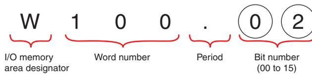
On the CX-Programmer, addresses in the CIO Area (including addresses for Serial PLC Links) are given with no I/O memory area designator. “CIO” is used as the I/O memory area designator in this manual for clarity.
