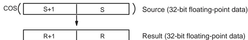
Specify the desired angle (-65,535 to 65,535) in radians in S+1 and S. If the angle is outside of the range -65,535 to 65,535, an error will occur and the instruction will not be executed. For information on converting from degrees to radians, see 3-14-9 DEGREES TO RADIANS: RAD(458).
