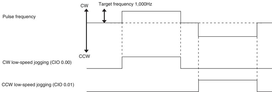
The example shows jogging with acceleration and deceleration executed using an ACC instruction. It is used for high-speed jogging.
