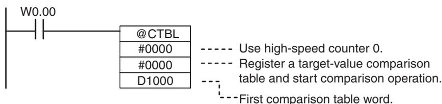
When execution condition W0.00 turns ON, the comparison starts with high-speed counter 0.
