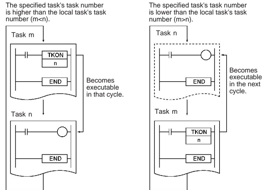
TKON(820) will be treated as NOP(000) if the specified task is already executable or the local task is specified.
