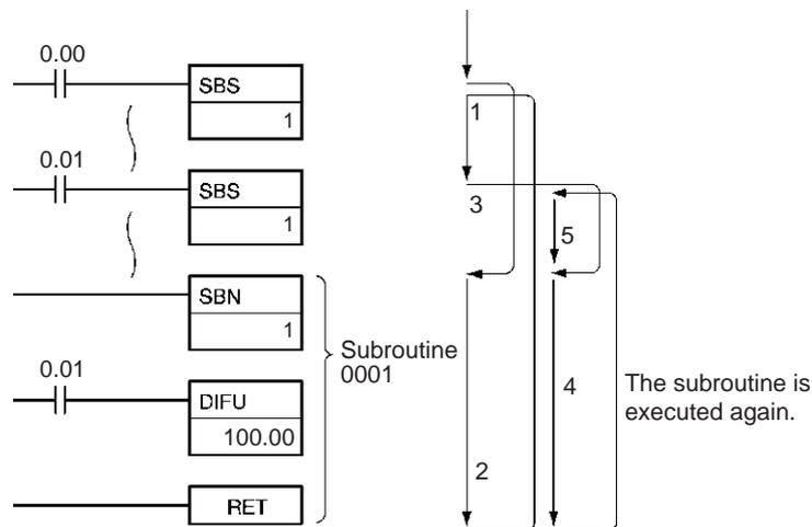
In contrast, the output of a differentiated instruction (DIFU(013) or DIFD(014)) would remain ON if the instruction was executed and the output was turned ON but the same subroutine was not called a second time.
