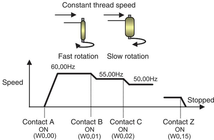
The target speed is changed according to inputs from multiple contacts. Acceleration and deceleration are controlled using the acceleration and deceleration of an inverter.
