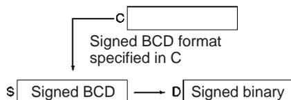
When the converted data is negative, it will be output as the 2's complement and the Negative Flag will be turned ON. NEG(160) can be used to determine the absolute value of a negative signed binary number. Refer to 3-11-5 2'S COMPLEMENT: NEG(160)395 for details.
