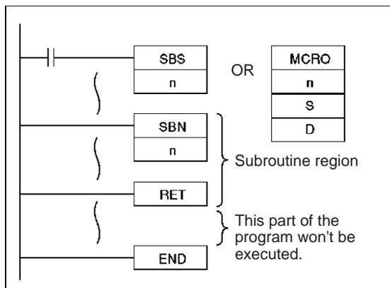
Be sure to place each subroutine in the same program (task) as its corresponding SBS(091) or MCRO(099) instruction. A subroutine in one task cannot be called from another task. It is possible to program a subroutine within an interrupt task.
