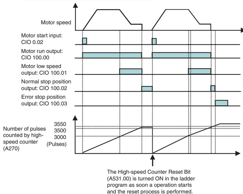
While the pulse count is between 3,500 and 3,550, normal stop position output (CIO 100.02) will be ON. If the pulse count exceeds 3,550, the error stop position output (CIO 100.03) will turn ON.
