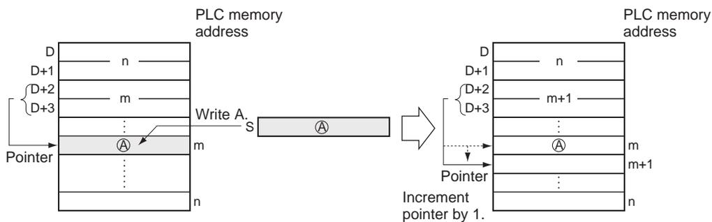
After PUSH(632) has been used to write data into a stack, FIFO(633) and LIFO(634) can be used to read data from the stack.
