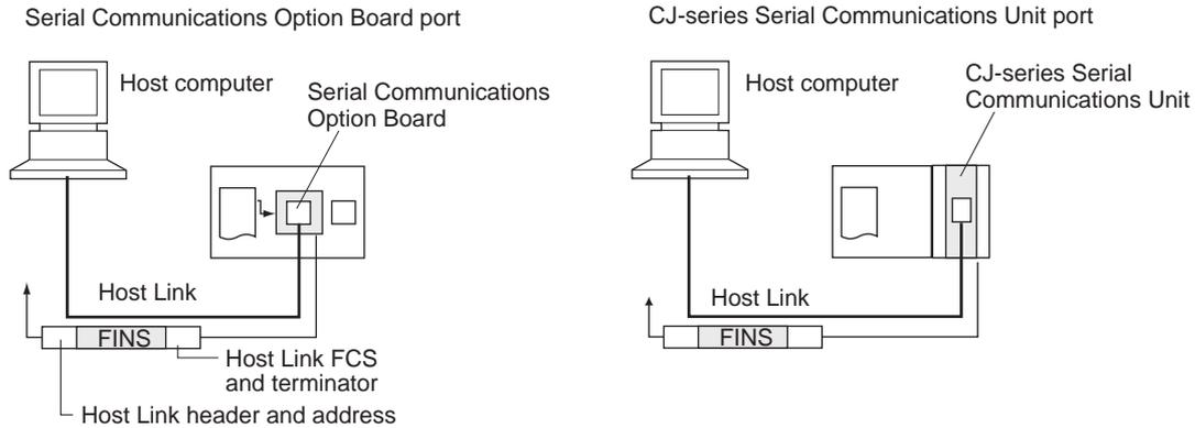
**Note** Host Link communications can be sent through the network. In this case, the FINS command travels through the network normally. When the command reaches the Host Link system, the necessary Host Link header and terminator are attached to the FINS command and the command is sent to the host computer.
