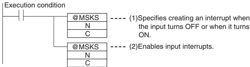
The MSKS instruction must be executed only once to make the settings, so in general execute MSKS in just one cycle using the upwardly differentiated variation of the instruction.
