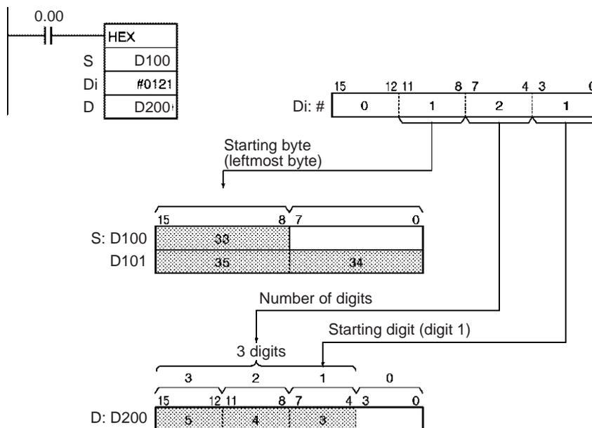
When CIO 0.00 is ON in the following example, HEX(162) converts the ASCII data in D100 beginning with the rightmost byte and writes the hexadecimal equivalents in D200 beginning with digit 1.
