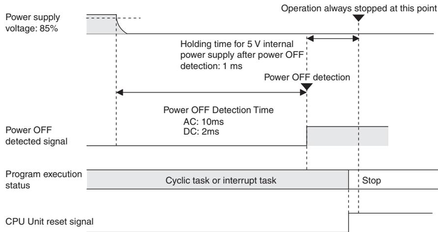
**Power OFF Detection Time:** The time from when the power supply voltage drops to 85% or less the rated voltage until the power interruption is detected.
