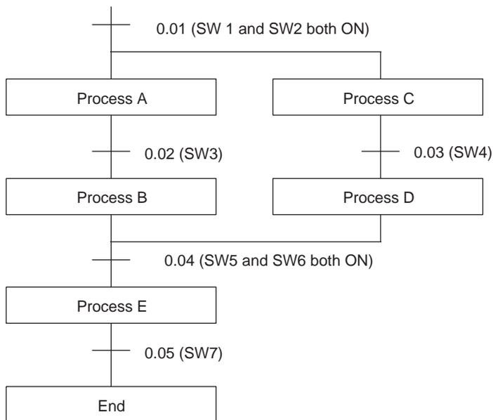
The program for this operation, shown below, starts with two SNXT(009) instructions that start processes A and C. These instructions branch from the same instruction line and are always executed together, starting steps for both A and C. When the steps for both A and C have finished, the steps for process B and D begin immediately.
