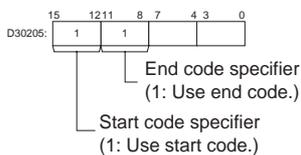
In this example, a start and end code have been specified in the allocated DM Setup
