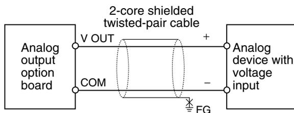
**Note 1** Separate wiring from power lines (AC power supply lines, high-voltage lines, etc.)
