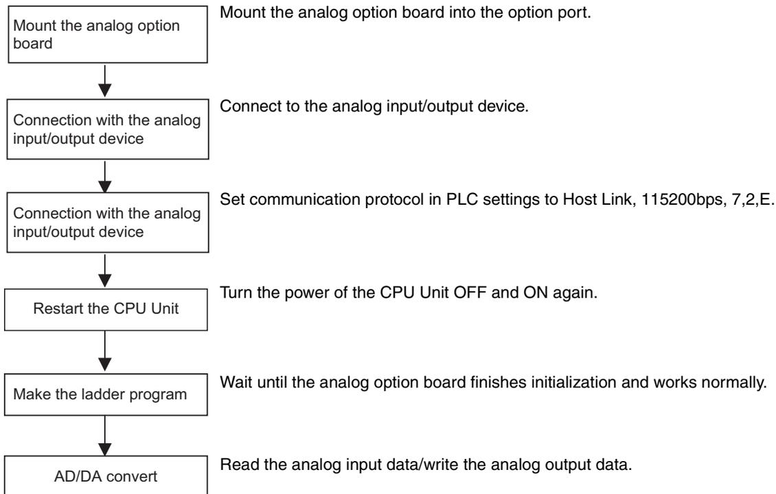
**Note 1** If PLC communication protocol setting is error, the option board will always try to link the PLC, and the error LED will be lit.
