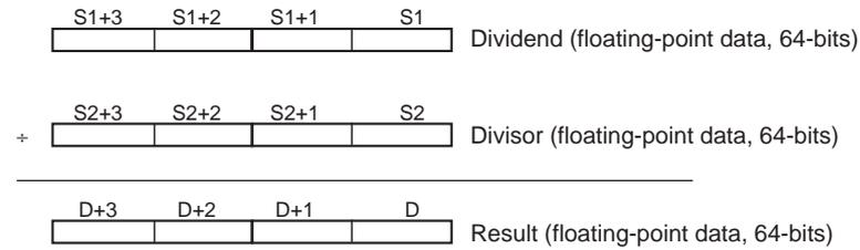
If the absolute value of the result is greater than the maximum value that can be expressed as floating-point data, the Overflow Flag will turn ON and the result will be output as  $\pm\infty$ .
