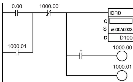
When CIO 0.00 is turned ON, 10 words are read from the Special I/O Unit with unit number 3, and are stored in D100 to D109.
