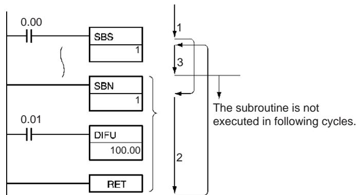
In the following example, subroutine 0001 is executed if CIO 0.00 is ON. Output CIO 100.00 is turned ON by DIFU(013) when CIO 0.01 has gone from OFF to ON. If CIO 0.00 is OFF in the following cycle, subroutine 0001 will not be executed again and output CIO 100.00 will remain ON.
