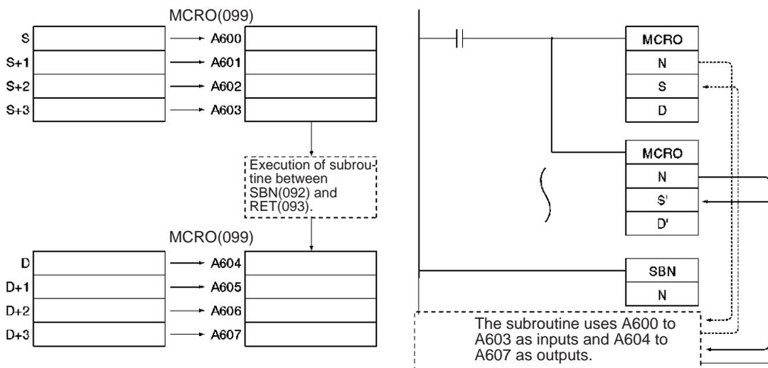
MCRO(099) can be used to consolidate two or more subroutines with the same structure but different input and output addresses into a single subroutine program. When MCRO(099) is executed, the specified input and output data is transferred to the specified subroutine.
