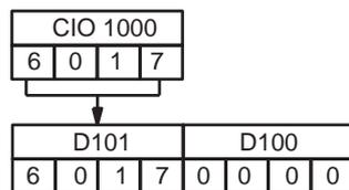
3. ROOT(072) calculates the square root of D101 and D100 and writes the result to D102.
