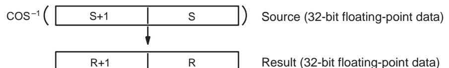
The source data must be between  $-1.0$  and  $1.0$ . If the absolute value of the source data exceeds  $1.0$ , an error will occur and the instruction will not be executed.
