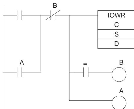
When the input condition is met, self maintenance is performed by output A and IOWR(223) is executed with each cycle until the Equals Flag turns ON. When the writing is completed and the Equals Flag turns ON, output B turns ON and the self maintenance is cleared.
