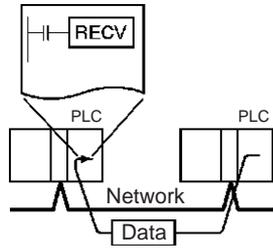
**Transmission from a Host Computer Connected through Host Link**
