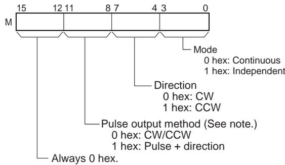
**Note:** Use the same pulse output method when using both pulse outputs 0 and 1 (CP1H only).
