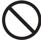
The circle and slash symbol indicates operations that you must not do. The specific operation is shown in the circle and explained in text.
