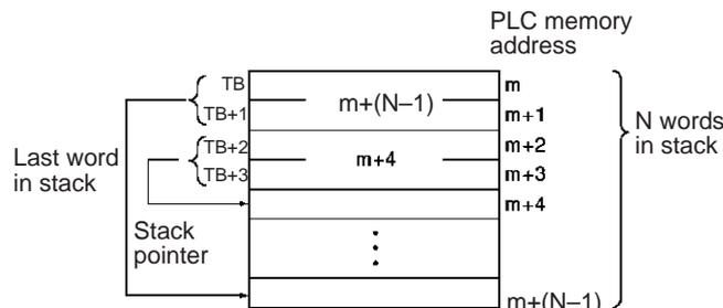
SSET(630) just establishes and initializes a stack. Use the following instructions to store in the stack and read data from the stack.
