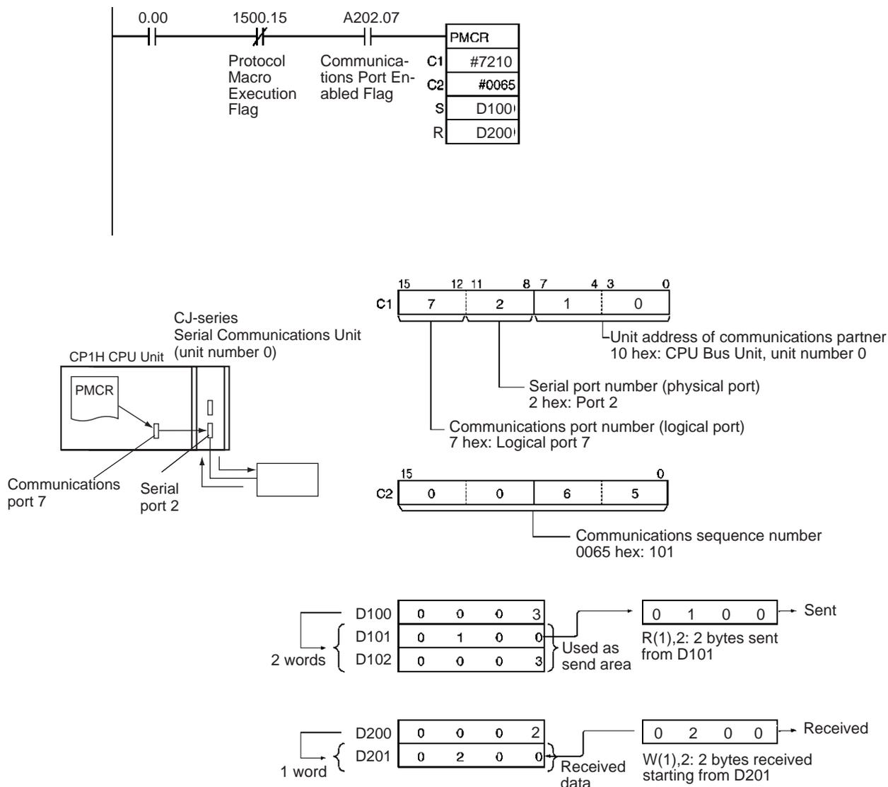
**Note** As shown above, the symbol read option, R( ), in the send message or the symbol write option, W( ), actually sends/receives data.
