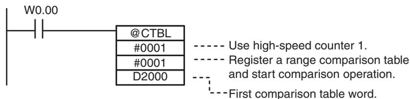
When execution condition W0.00 turns ON, the comparison starts with high-speed counter 1. When the PV of high speed counter 1 is between 25,000 and 25,500, cyclic task execution is interrupted, and interrupt task 12 is executed. When interrupt task 12 execution is completed, execution of the interrupted cyclic task resumes.
