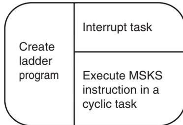
Write the program in the interrupt task. Interrupt tasks 2 to 7 correspond to interrupt inputs 2 to 7.
