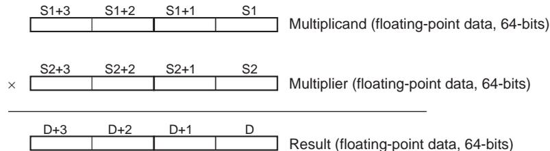
If the absolute value of the result is greater than the maximum value that can be expressed as floating-point data, the Overflow Flag will turn ON and the result will be output as  $\pm\infty$ .
