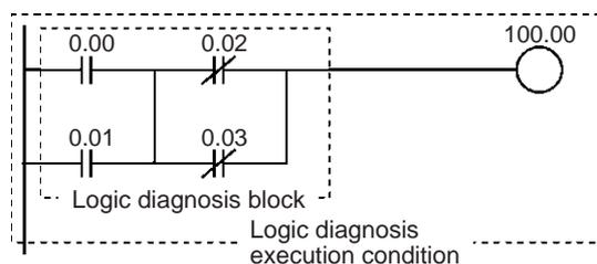
The logic diagnosis function is executed every cycle as long as the execution condition for FPD(269) is ON. The operation of the logic diagnosis function is independent of the time monitoring function.
