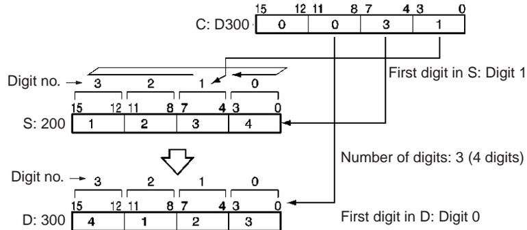
**Note** After reading the leftmost digit of S (digit 3), MOVD(083) wraps to the rightmost digit (digit 0).
