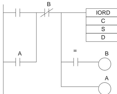
When the input condition is met, self maintenance is performed by output A and IORD(222) is executed with each cycle until the Equals Flag turns ON. When the reading is completed and the Equals Flag turns ON, output B turns ON and the self maintenance is cleared.
