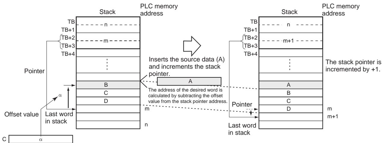
SINS(641) can be used to insert the data for an item that is inserted in the midst of items already on a conveyor. The position of the insertion point is simply the number of items back (the offset value) from the most recent item added to the conveyor.
