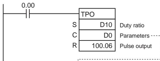
TPO(685) takes the duty ratio in D10, converts that duty ratio to a time-proportional output, and outputs the pulse output to bit 00 of CIO 100.06.
